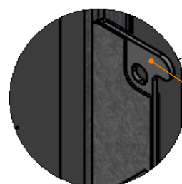
D01.04510.03 Dividers to secure the displays and prevent them from moving side to side.
